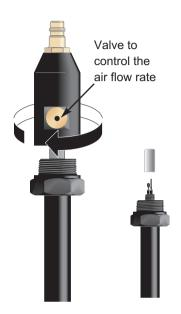
Place the measuring chamber on the humidity probe adapter and screw on tightly by hand.
